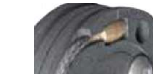
Fig.31 : assembled drive wire in a tensionable drive wheel
