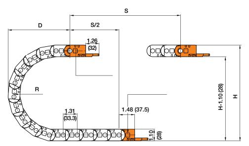
is measured from the center of the curve loop to the center of the pivot pin on the side link. Do not confuse bend radius with the dimension of the overall curve height!
