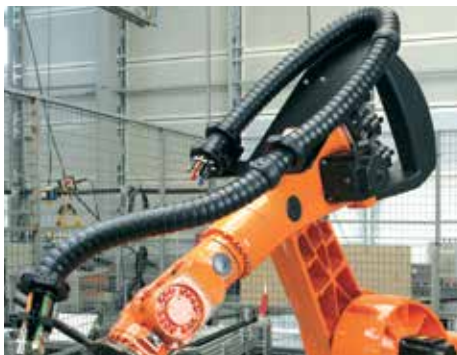
triflex® RS for a lean e-chain® guide. Integrated spring rods generate the directed pretension so that loops do not form in the working area
