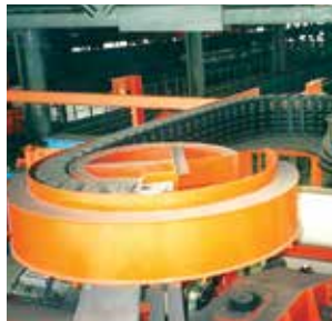
Rotary motion of 180° with a standard e-chain® on a crane turret drive
