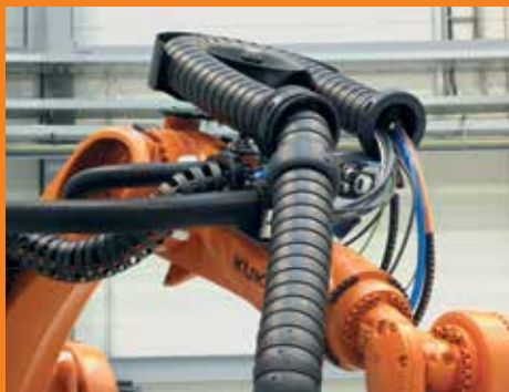
Close routing on the robot arm without loop formation
