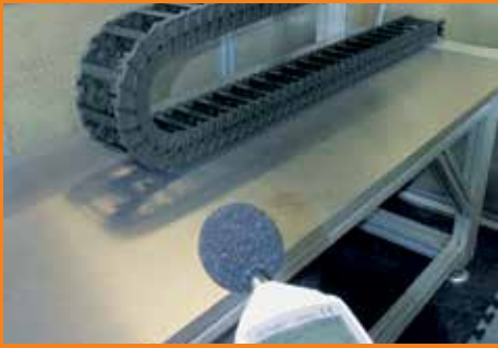
Noise level test inside an igus® acoustic cell
