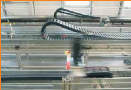
Speed up to 10 ms and acceleration up to 656 ft/s 2 are tested by igus®
