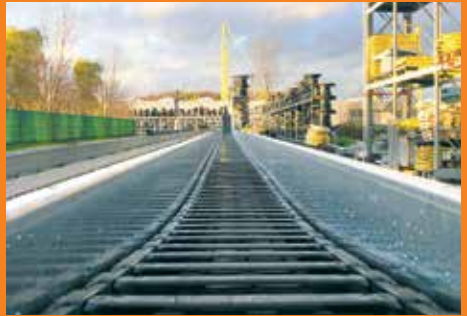
Long travel test field - 125 m travel length, speed 984 ft/min
