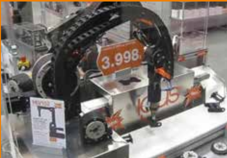
Trade fair machine – 5 DOF robot arm with RL-D and RL-S joints. System simulates real use in the igus® factory (igus®)
