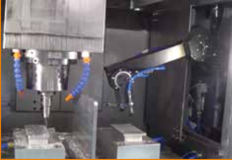
robotlink® D – Suction arm in a machine tool (igus®)
