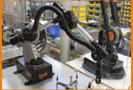
Trade fair machine RL-DQ-RBT-5532S-AC with 5 DOF and 3-finger gripper (igus®)
