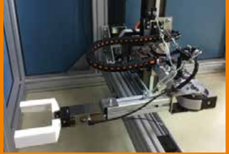
Storage and retrieval unit with two RL-D and drylin® linear guides (MATRIUM GmbH)
