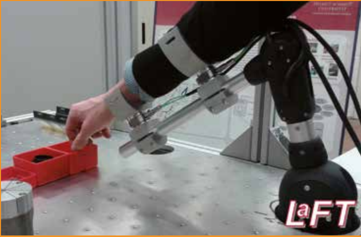
Manual workstation support system with human-machine interface for the production of the Manufacturing Technology Lab (LaFT) at Helmut-Schmidt University in Hamburg
