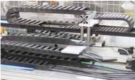
CFLG-2LB-50/125 tested with 70.4 million strokes at 4.35 x d
