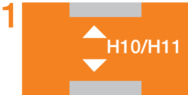
Poor tolerance of punched housing or drawn sheet metal
