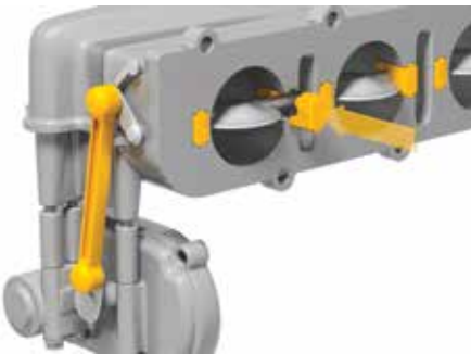
Active intake manifolds
