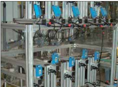
Pivot wear test rig for testing the pivoting wear rate for medium loads
