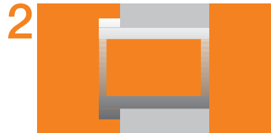
Assembly of iglide® bearing with transition fit
