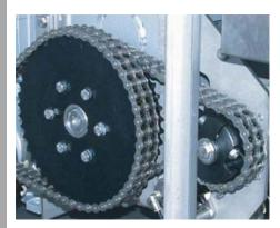
The enormous increase in service life - without maintenance - for the roller chain is due to its special joint structure. A high-performance iglide® plastic bushings from igus® was integrated and significantly enhance the tribology of the chain joint. The iglide® bushings distinguish themselves with an extremely high wear resistance, low coefficient of friction, high compressive strength, as well as chemical resistance. In addition, they are maintenance-free and insensitive to dirt.
