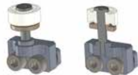
The custom sliders allow the (small) weight of the door to slide along the custom non-linear track and ball bearings help constrain the door within these tracks. This allows for defining some interesting motion paths, as long as driving linkage can be found to complement it.
